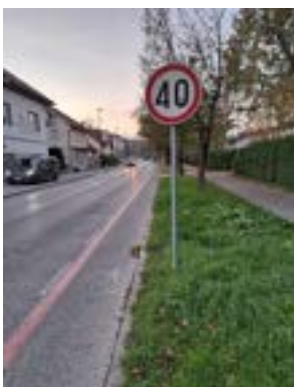
Marked bicycle lanes on the carriageway where the speed limitation exceeds 30 km/h (Photo LKM)
